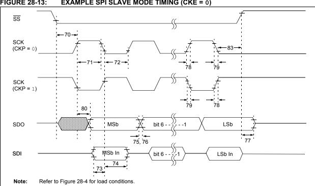
FIGURE 28-13: **EXAMPLE SPI SLAVE MODE TIMING (CKE = 0)**
