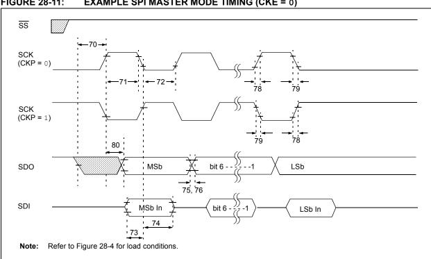
**FIGURE 28-11: EXAMPLE SPI MASTER MODE TIMING (CKE = 0)**
