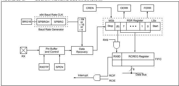
FIGURE 20-7: ASYNCHRONOUS RECEPTION, RXDTP = 0 (RX NOT INVERTED)
