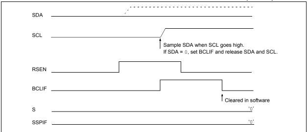
FIGURE 19-32: BUS COLLISION DURING REPEATED START CONDITION (CASE 2)
