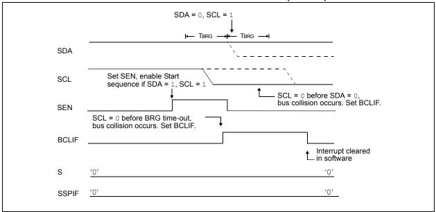
FIGURE 19-30: BRG RESET DUE TO SDA ARBITRATION DURING START CONDITION
