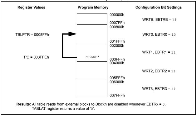
FIGURE 25-8: EXTERNAL BLOCK TABLE READ (EBTRx) ALLOWED
