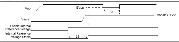
TABLE 28-12: RESET, WATCHDOG TIMER, OSCILLATOR START-UP TIMER, POWER-UP TIMER AND BROWN-OUT RESET REQUIREMENTS
