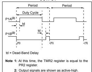
FIGURE 16-5: EXAMPLES OF HALF-BRIDGE OUTPUT MODE APPLICATIONS
