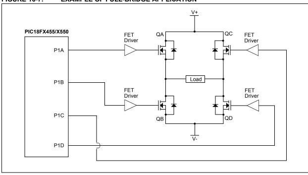
FIGURE 16-7: EXAMPLE OF FULL-BRIDGE APPLICATION
