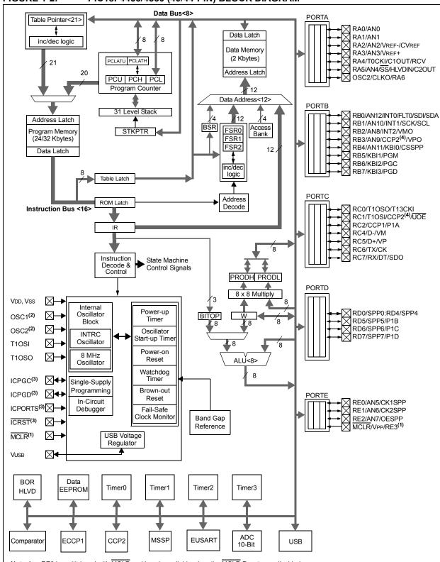
FIGURE 1-2: PIC18F4455/4550 (40/44-PIN) BLOCK DIAGRAM
