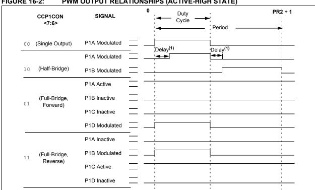
**FIGURE 16-2:** PWM OUTPUT RELATIONSHIPS (ACTIVE-HIGH STATE)
