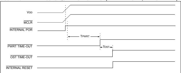
FIGURE 4-4: TIME-OUT SEQUENCE ON POWER-UP (MCLR NOT TIED TO VDD): CASE 1
