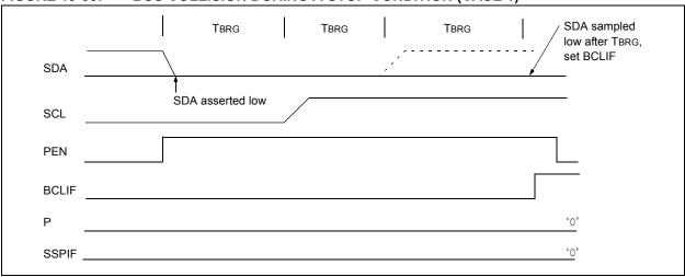
FIGURE 19-34: BUS COLLISION DURING A STOP CONDITION (CASE 2)
