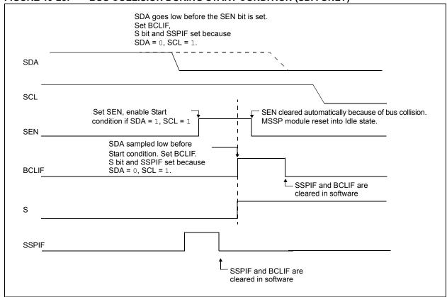
FIGURE 19-29: BUS COLLISION DURING START CONDITION (SCL = 0)
