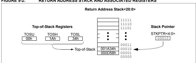
FIGURE 5-2: RETURN ADDRESS STACK AND ASSOCIATED REGISTERS
