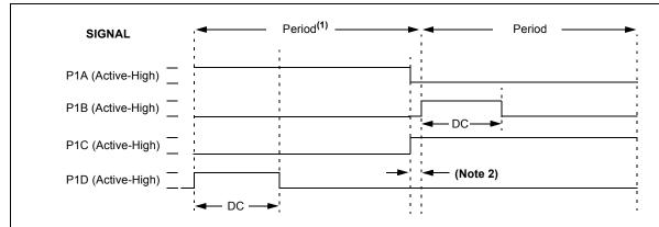
Note 1: The direction bit in the CCP1 Control register (CCP1CON<7>) is written any time during the PWM cycle.
