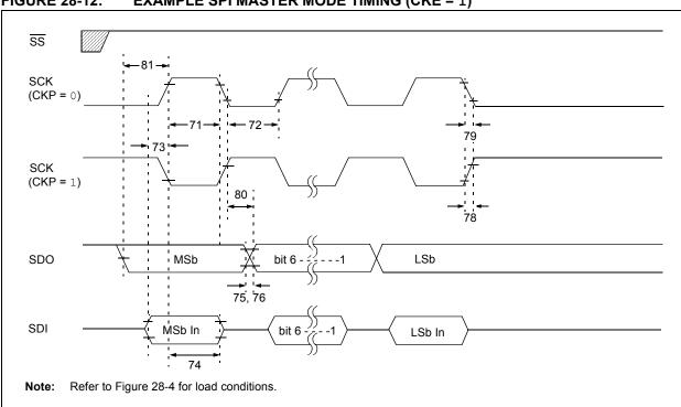
FIGURE 28-12: **EXAMPLE SPI MASTER MODE TIMING (CKE = 1)**
