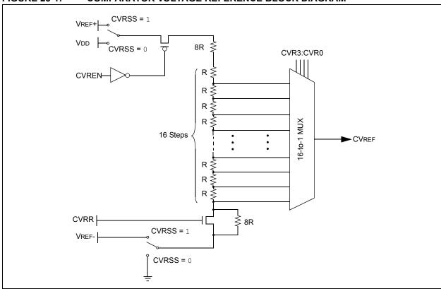
FIGURE 23-1: COMPARATOR VOLTAGE REFERENCE BLOCK DIAGRAM
