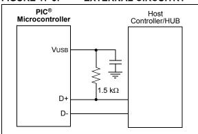
Note: The above setting shows a typical connection for a full-speed configuration using an on-chip regulator and an external pull-up resistor.
